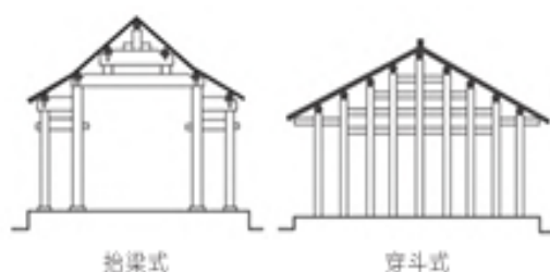
Figure 10: Post and lintel construction and column and tie construction (Su et al., 2023)
