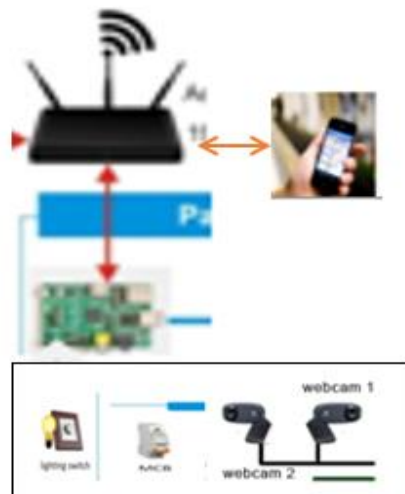
Figure 4. Local Network Architecture
